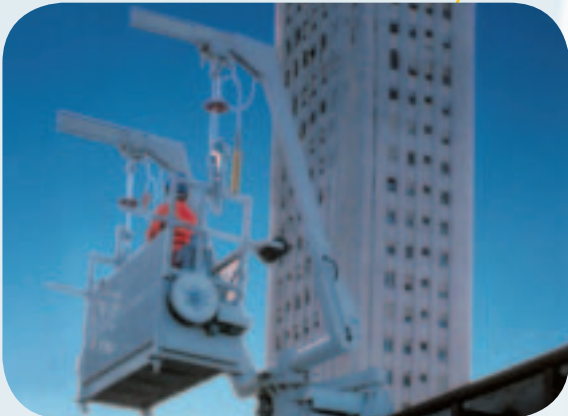
Cradle suspended from parapet mounted powered trolley
